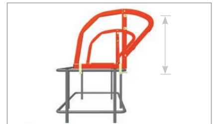
660mm high for optimal operator protection
