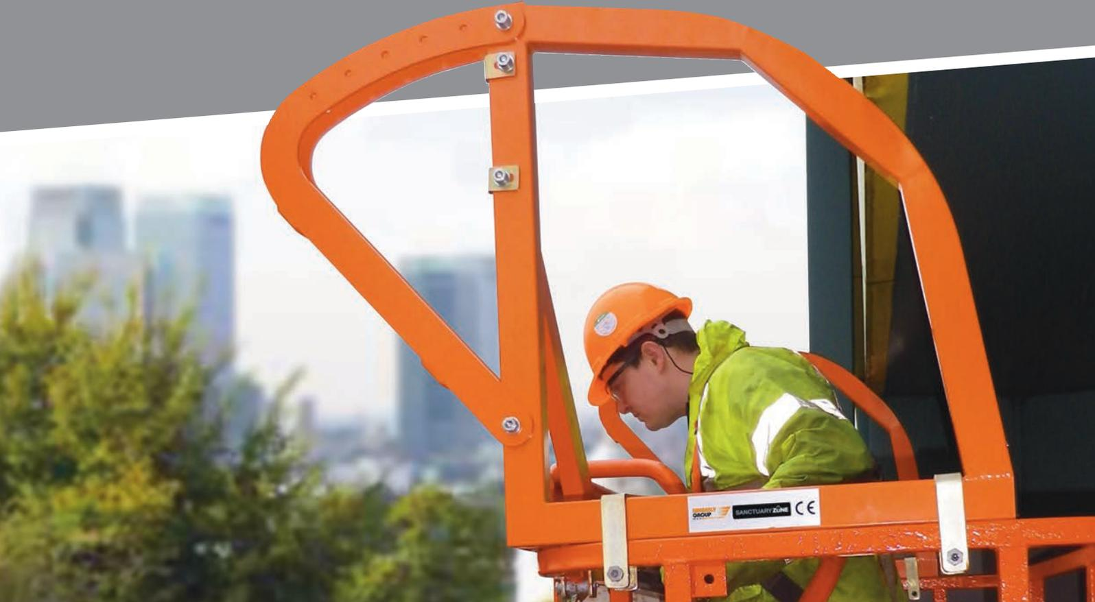
**Being crushed against overhead obstructions, resulting in death or serious injury, is one of the main hazards facing operators of Mobile Elevating Work Platforms (MEWPs).**
